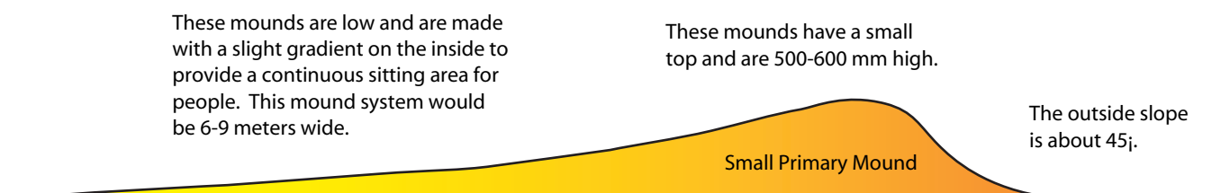
Figure 2: After Shaping the Mound System
