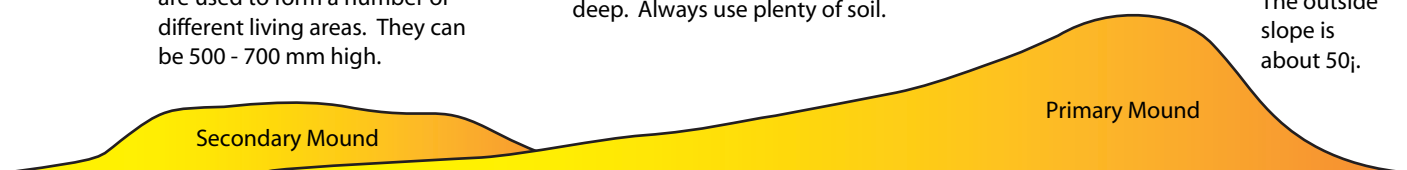
Figure 2: After Shaping the Mound System
