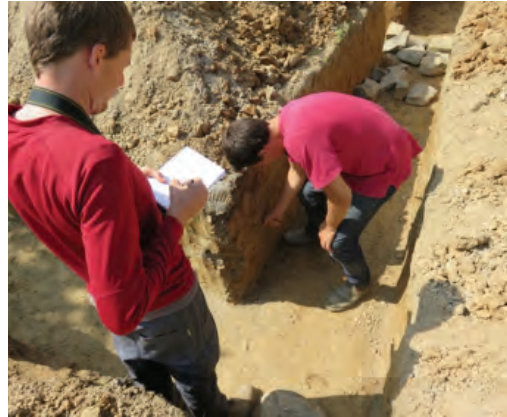
Undertaking pencil test to determine stability of foundations
