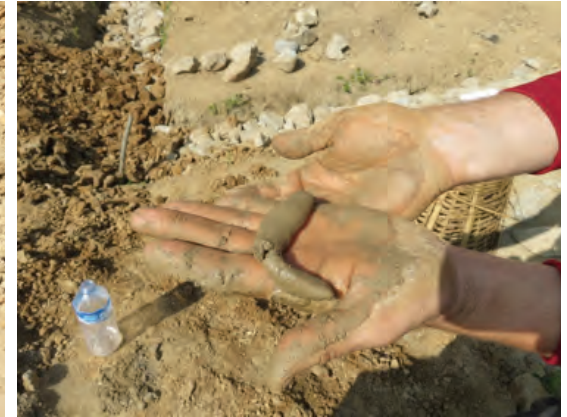
Testing clay content of soil for use in mortar
