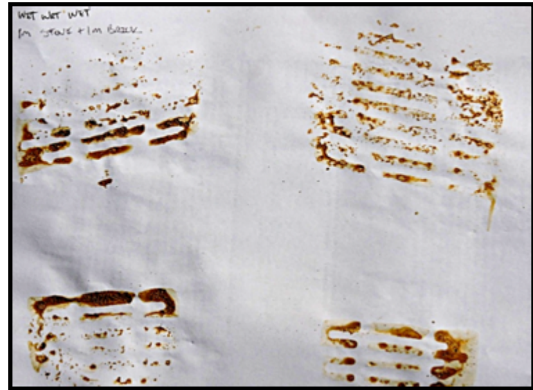
6'(1800) mud + 3' (900) stone + 3' (900) brick = dry Less mud in the toilet area
