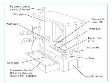
Figure 7. Key components of a composting toilet
