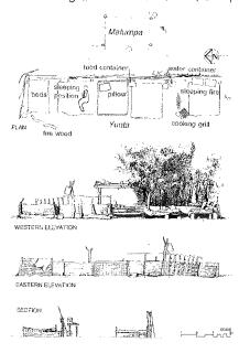
Figure 2. A plan, sections and elevations describing a Warlpiri yunta in a jilimi (women's residence) that was documented during May 1994 in Nyirripi, a settlement located approximately 350 kilometres west of Alice Springs. [Source: Keys, 1999, Fig.41. Artist: C. Keys.]
