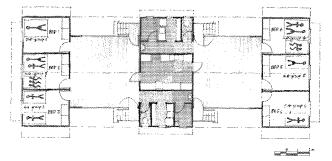
Figure 5 A house built at Ngukurr (Roper River, N.T.) during 1998-99 and designed to accommodate a complex Indigenous household. The household genealogy and floor plan show the sleeping locations of the six household subunits or groups. The total population of the household was 14. [Architects, Northern Building Consultants, Darwin, Source: Memmott et al, 2000.]
