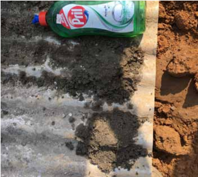
Use of detergent tested to increase runniness of mortar but deemed unnecessary
