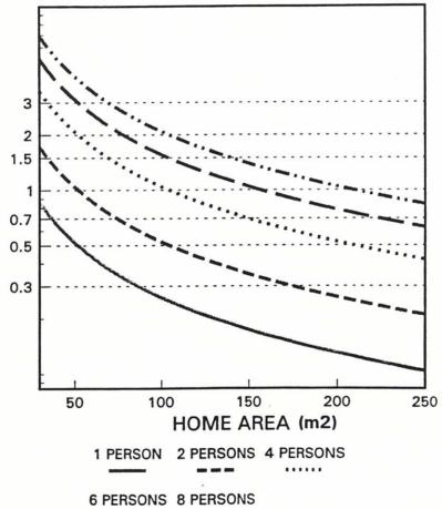
Basic calculations with 30% extra ventilation to achieve sufficient ventilation with varying habits with relation to humidity production
