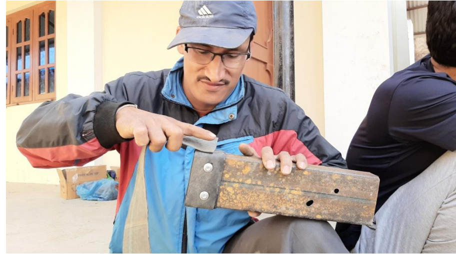
Making of door stopper for the first toilet doors at Panchakanya Basic School
