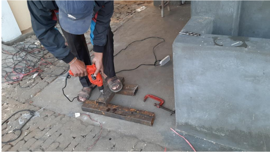
Making of door stopper for the first toilet doors at Panchakanya Basic School
