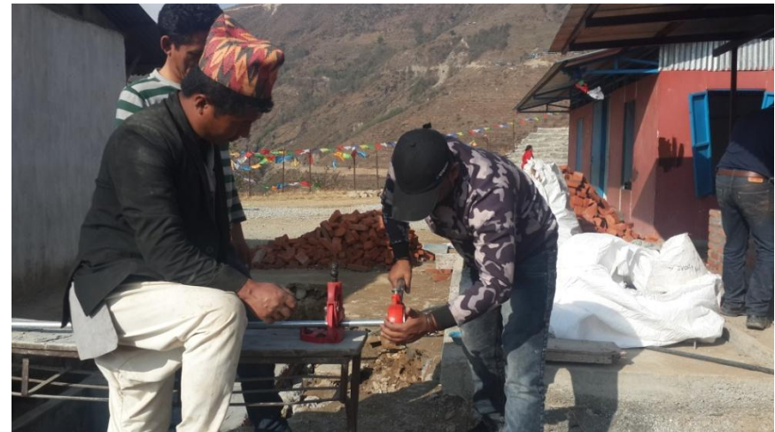
Teaching Jale Tamang – How to make threading on GI pipe.
