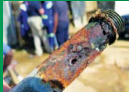
FIGURES 23: Water metres were installed (which required new galvanised pipes due to deterioration) and systems for regular readings were established.
