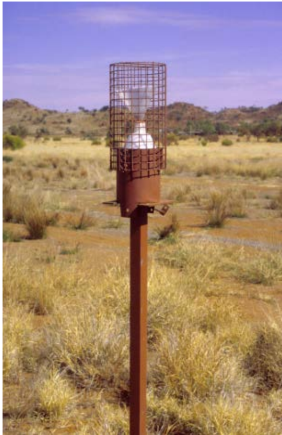
LEFT Typical simple dust monitor located in a predetermined grid around the village
