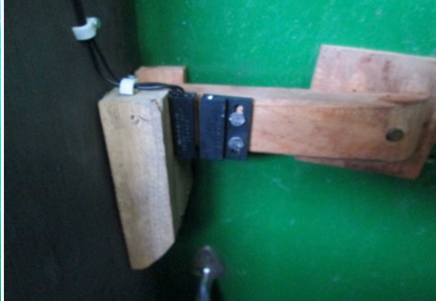
The inside lock in the closed position and the magnetic reed switch stores the event and duration into the data logger for future download
