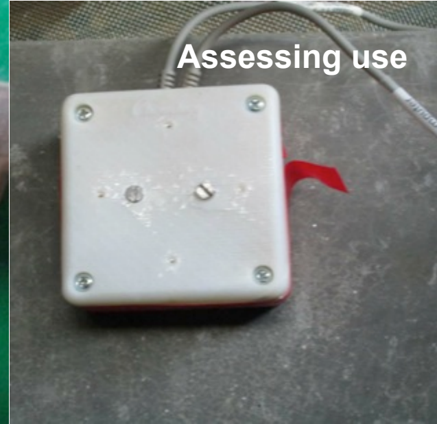
The inside lock in the closed position and the magnetic reed switch stores the event and duration into the data logger for future download
