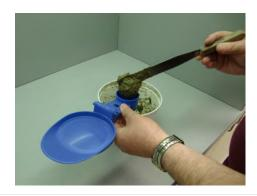
5. Let the mixture dry sufficiently. The dried counterweight should weigh around 140g.
