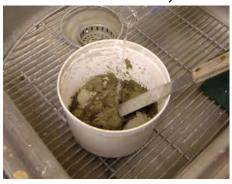
4. The counterweight mixture should weigh around 150g when filled to the top of cup.
